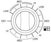
Continuing to turn counter-clockwise will bring you into the HI setting for the two inner elements combined. From here, continue turning counter-clockwise to go into the MED, and LOW settings of both elements.
